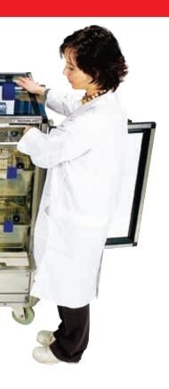
The IVC Recovery Unit is a Tecniplast product designed to ensure a controlled temperature and ventilation environment for animals during post-surgical treatment and isolation of selected weak/sick groups of animals for Veterinary inspection or treatment.
