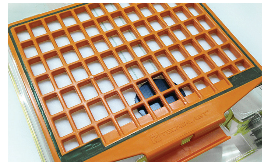
Filter top with RFID tag for cage identification and location
