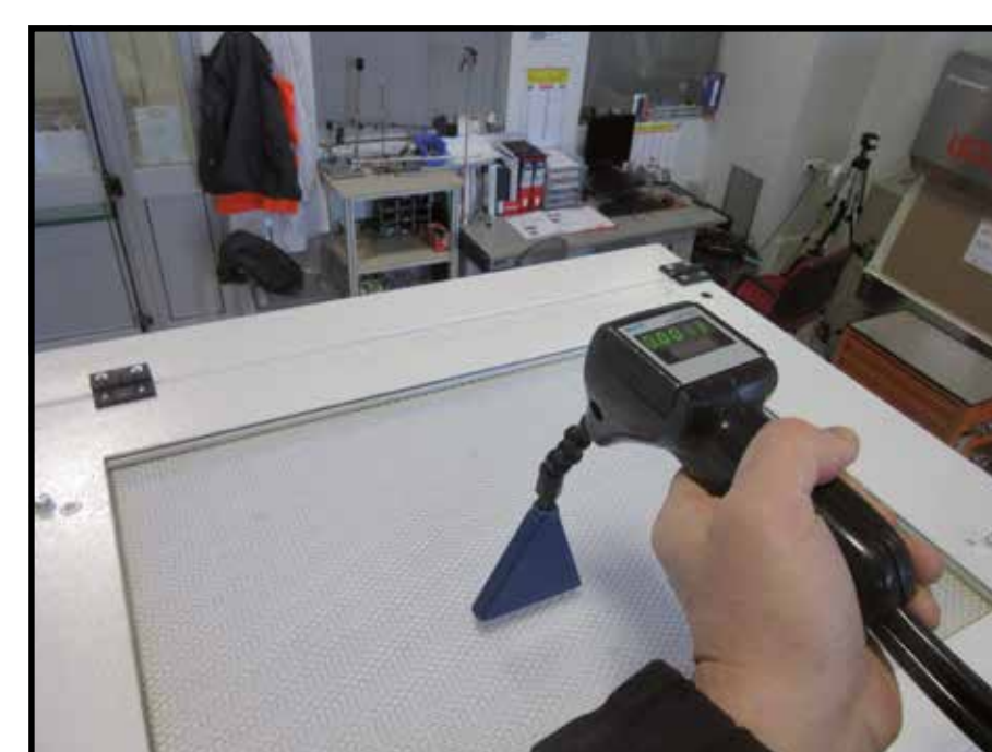
Fig.4 Scanning probe of the exhaust HEPA Filter.
