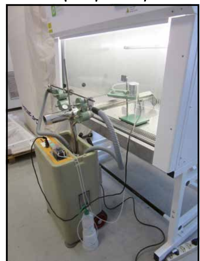
Fig.2 - KI-Discus Test for the retention efficiency at the front aperture.
