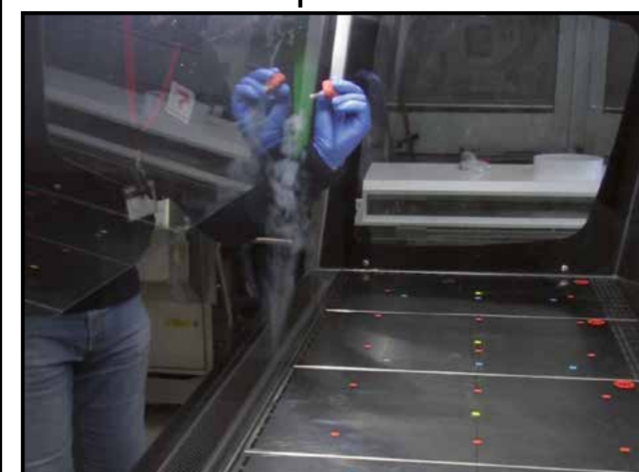
Fig.5 Smoke test for view screen retention test.
