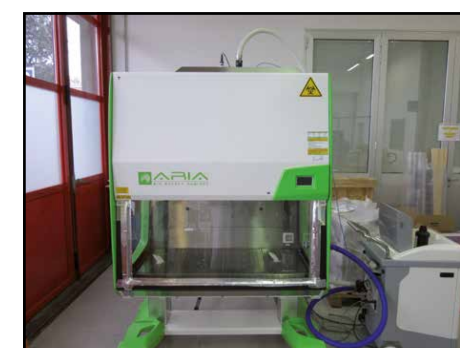
Fig. 6 - H 2 O 2 "In loop" Decontamination by Vaporized Hydrogen Peroxide System.
