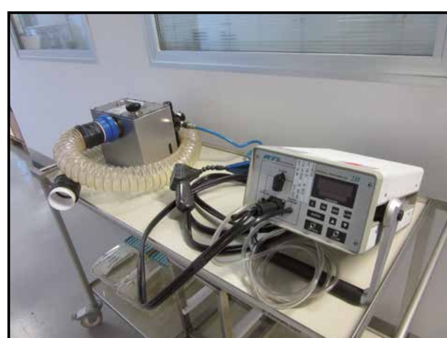
Fig.3 Aerosol generator and Photometer.
