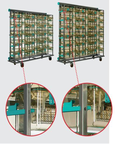
The vertical design of the exhaust plenums allows particles extracted from the cage (food, bedding, dander, debris, etc ...) to fall by gravity into the removable horizontal exhaust plenum. The removal of the horizontal supply and exhaust plenums is totally tool-free and can be easily performed by a single operator.
