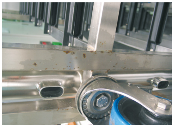
Fig. 9-7: View of stainless steel racks with corrosion
