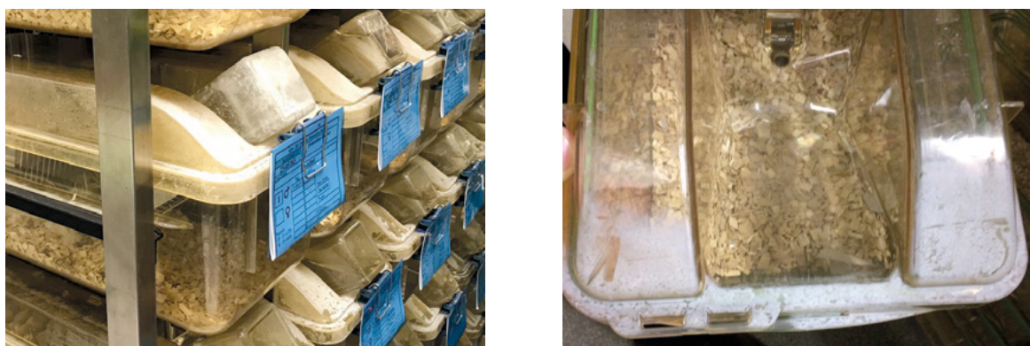
Fig. 9-2: left Cage top and drinking bottle made of polysulfone with milky white looking material clouding, right detailed view of cage bonnet
