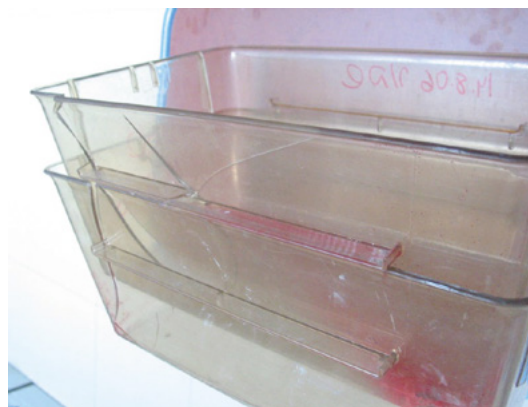
Fig. 9-6: Deformation of cage bases on the left, cracks in cage shells on the right
