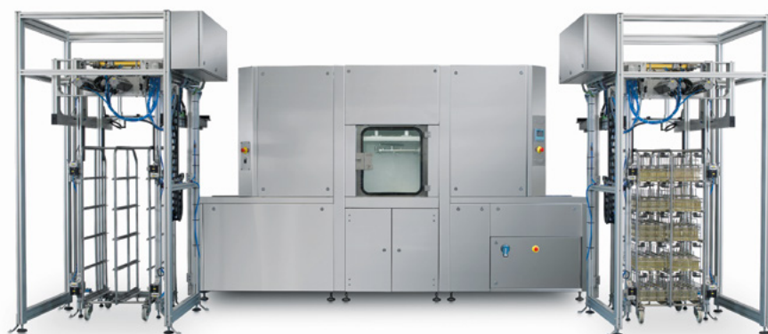
Figure 4-15: Bottle cleaning system with automatic loading of the bottle cages from a transport trolley, decapping, conveying, cleaning, filling, capping and automatic unloading of the bottle cages back into a transport trolley
