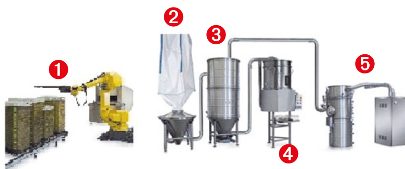
Fig. 4-20: Example of a fully automatic system: Filling the cages with robots or automatic machines (1), filling funnel for clean bedding, e.g. with BIG-Bag (2), optional storage silo (3), dosing funnel with dust extraction device (4) and vacuum generator and dust filter (4) for pneumatic conveying.
