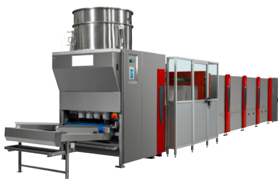
Fig. 4-19: Example of a fully automatic system: Bedding filling of automatically turned cage bases after cleaning in a cage belt cleaning system
