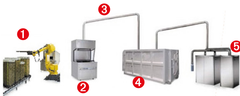
Fig. 4-8: Example of a fully automatic system: Emptying of the cage bases by robot or automatic machine (1) into the discharge hopper (2), with pneumatic conveying via pipework (3) into an external container (4); vacuum generator and dust filter (5)
