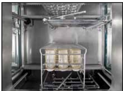
Single-nozzle bottle and cap wash pattern processed in separated layers
