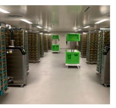
biowaste to inactivate liquid effluents and autoclave and SAS sterilization equipment to decontaminate products and materials before they leave this biosafety area. Inside we have three test laboratories and a housing room **for 1,000 cages in negative pressure IVC, as well as biological safety cabinets** to handle these rodents. This whole area occupies 200 m<sup>2</sup> with another 200 m<sup>2</sup> of technical floor.
