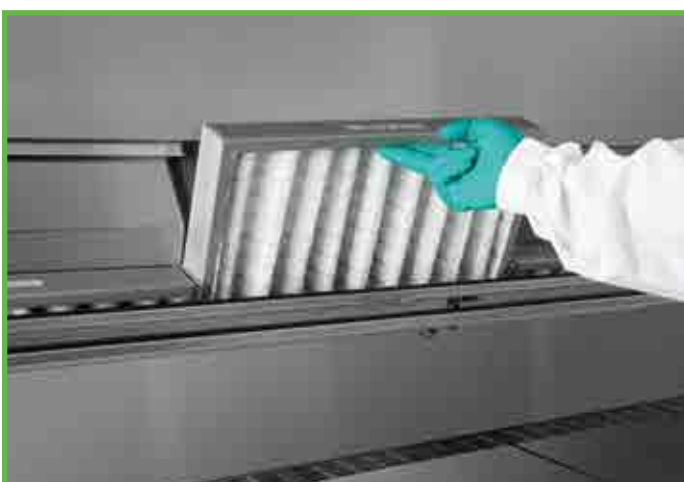
ERGONOMIC ACCESS TO PREFILTERS FOR EASY MAINTENANCE
