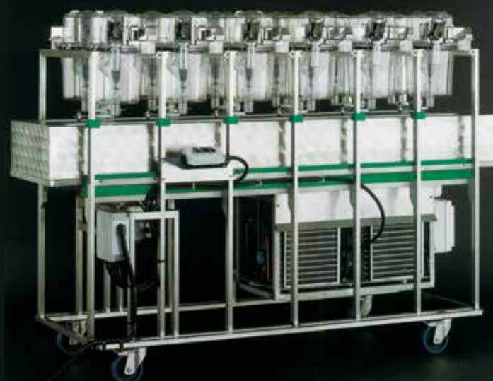
REFRIGERATED RACK FOR FRACTIONATED URINE COLLECTION
