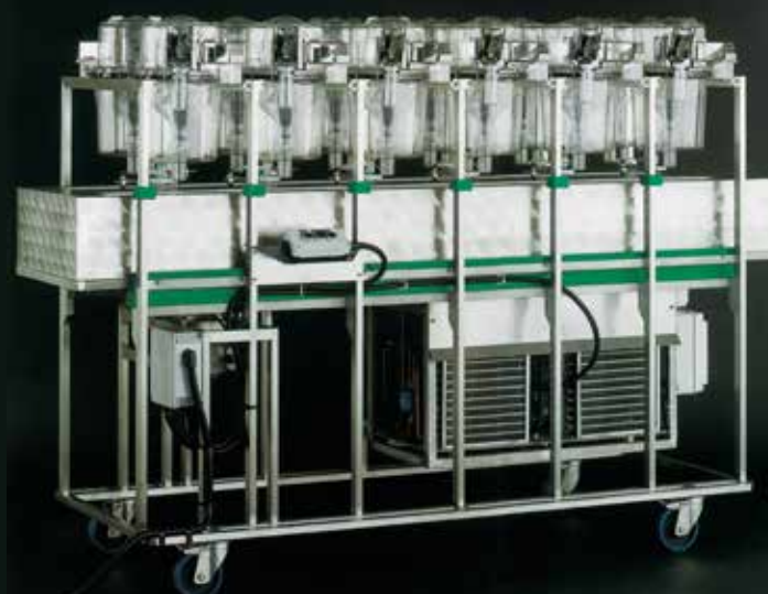
REFRIGERATED RACK FOR FRACTIONATED URINE COLLECTION
