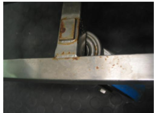
Figure. 9-5 Siphon and stainless steel rack with corrosion
