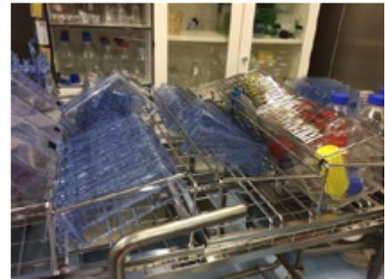
Fig. 3-1: Examples of how to load a cleaning station from practical experience
