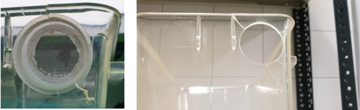
Figure. 9-2 Tank parts with stress cracks
