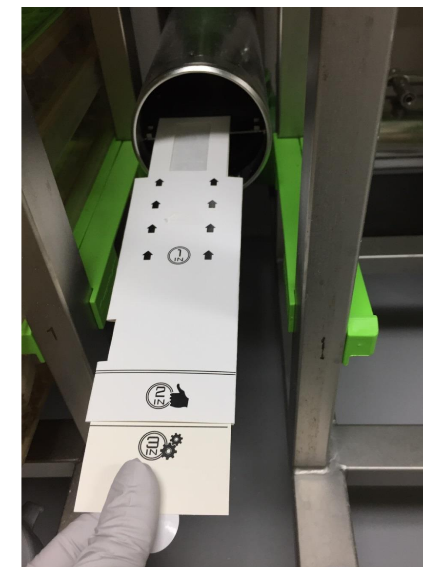
Figure 4. Interceptor being placed into the plenum attachment.
