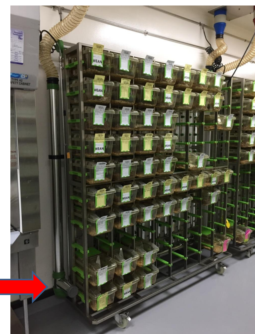
Figure 1. Two racks were fitted with a prototype plenum attachment to perform EAD testing (red arrow).
