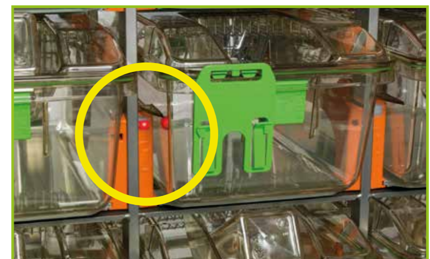
When the DVCTM detects a cage that needs attention, a LED light located in the runner turns-on to identify the cage.
